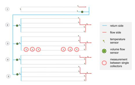
Fig. 3: Measurement setup of the volume flow and temperature sensors
