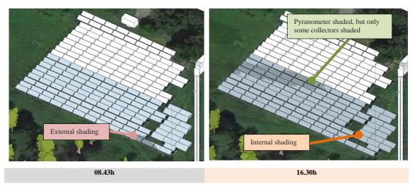
Fig. 4: Irradiance analysis of the test plant (2017-09-27)
