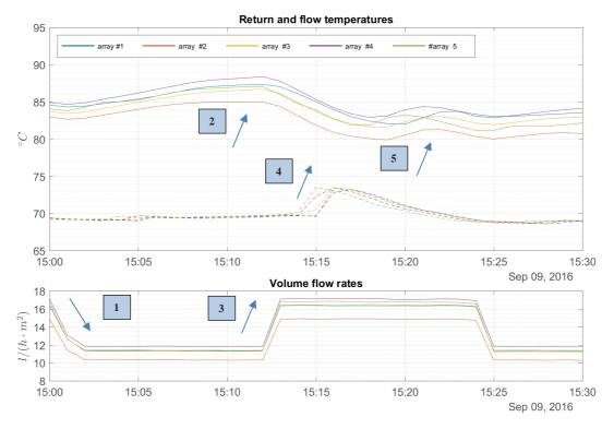
Fig. 5: Delayed response of the collector array outlet temperature (2, 5), when swift changes of the volume flow rate (1, 3) and return temperature (4) occur. Depicted are five arrays of the test plant.
